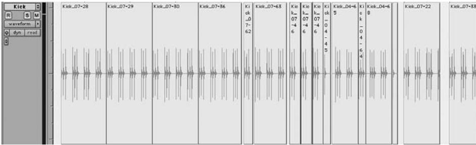
**Figure R.4** Each of the blocks on this track containing a waveform is a separate region of audio.
