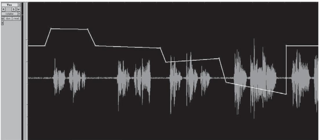
**Figure A.9** An automation curve represents the automation data recorded or entered into a track. Here we see a curve that will control the track’s volume fader.
