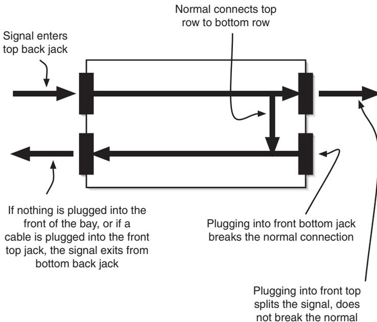
**Figure N.4** Plugging a jack into the top front jack on a half-normalised patch bay will result in a signal split. Plugging into the lower front jack interrupts the signal.
