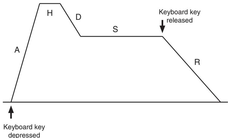
**Figure A.5** An AHDSR adds a fifth hold stage to the standard ADSR envelope.
