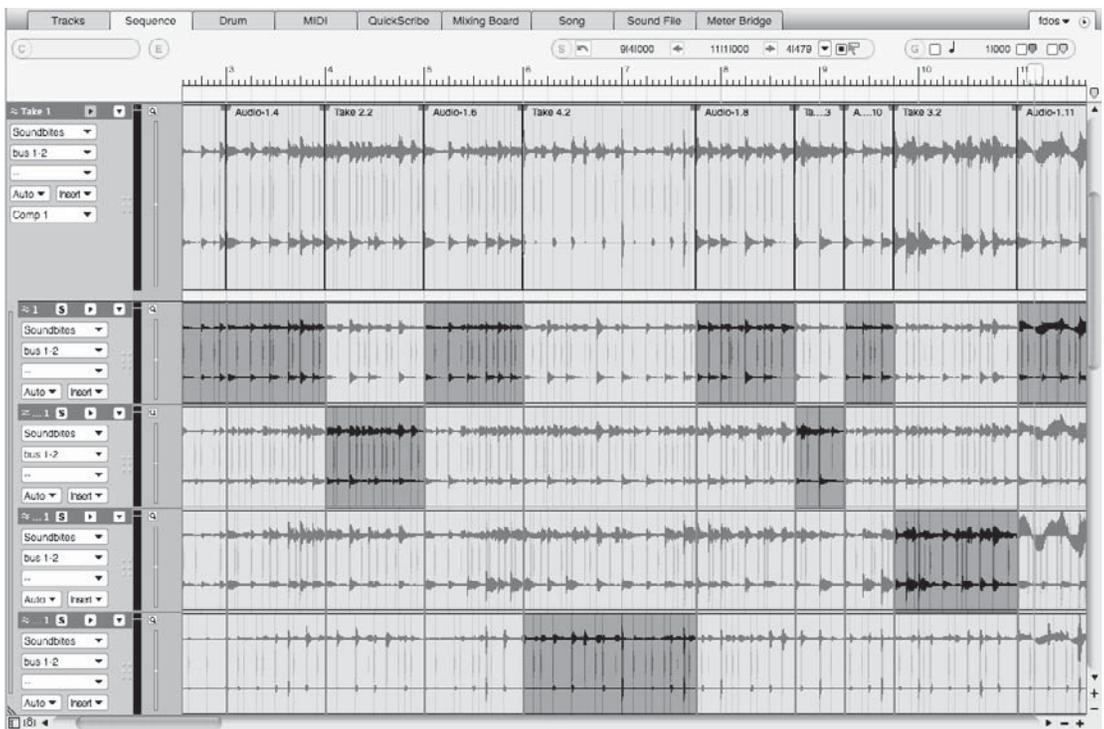
**Figure C.6** Comping is the process of combining the best parts of two or more tracks to make a new composite track. In this example, the top track is the “comp,” which has been created using the best parts of the four tracks below.
