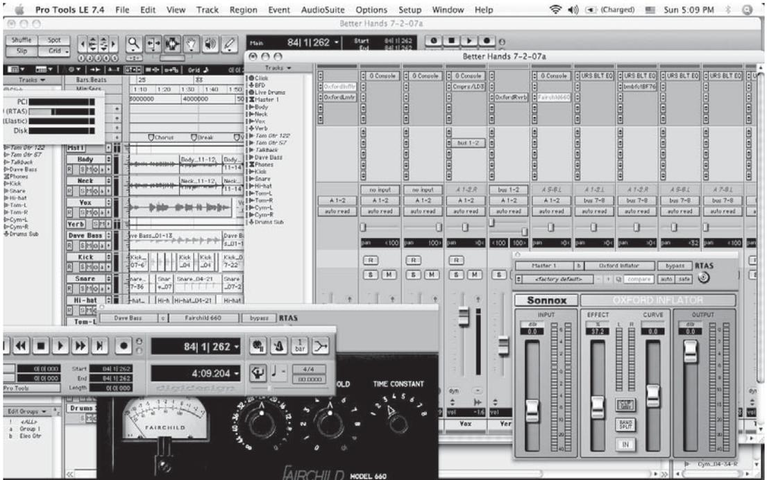
Figure D.2 A DAW can record, process, edit, mix, and play back audio.
