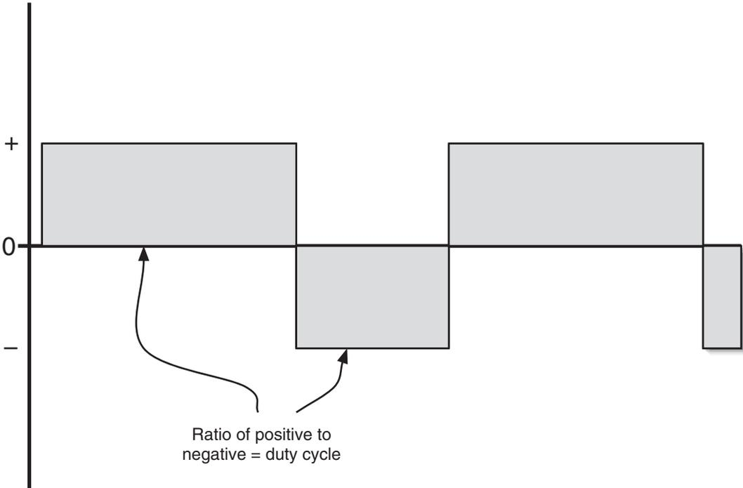
**Figure D.10** The duty cycle of square or rectangular wave is how long the wave is positive versus how long it is negative.
