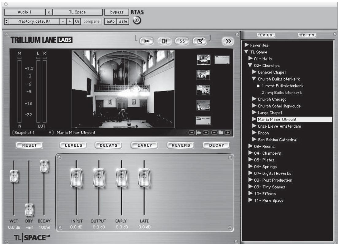
**Figure I.1** A convolution reverb such as Trillium Lane Labs, TL Space can use an impulse response created from the sound of a real room to add reverb to a track or signal.
