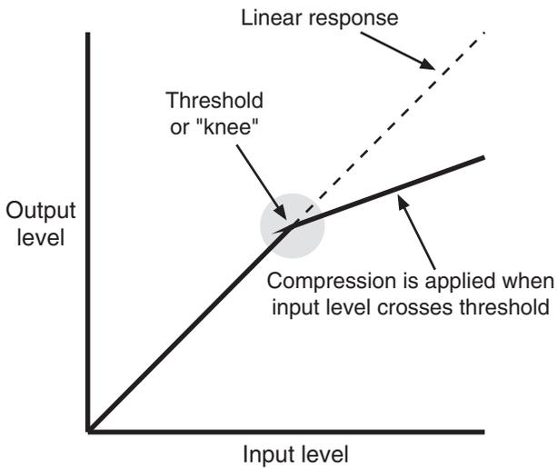
**Figure K.1** The knee is the point in a dynamics processor where the response changes—where compression begins to be applied.
