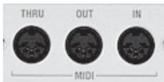
**Figure M.5** There are three types of MIDI ports or jacks: MIDI inputs, MIDI outputs, and MIDI thrus.
