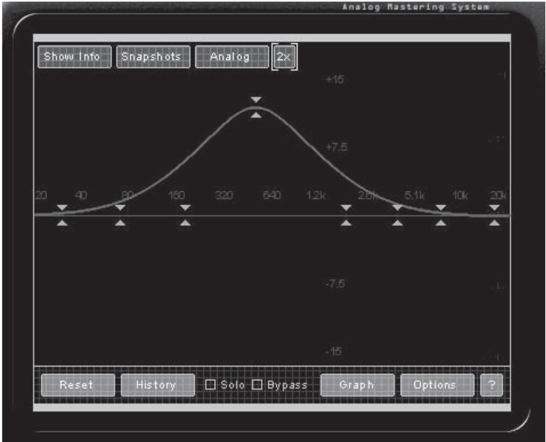
**Figure B.7** Bell filters have a response curve that resembles the basic bell curve when boosting or cutting.
