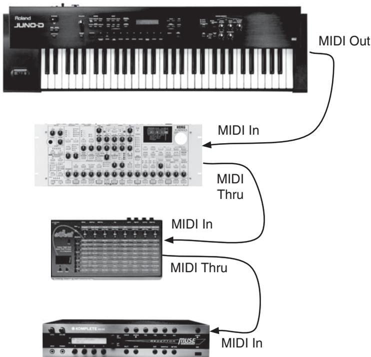
**Figure D.1** MIDI equipment is often connected together in daisy-chain fashion, MIDI thru to MIDI input.
