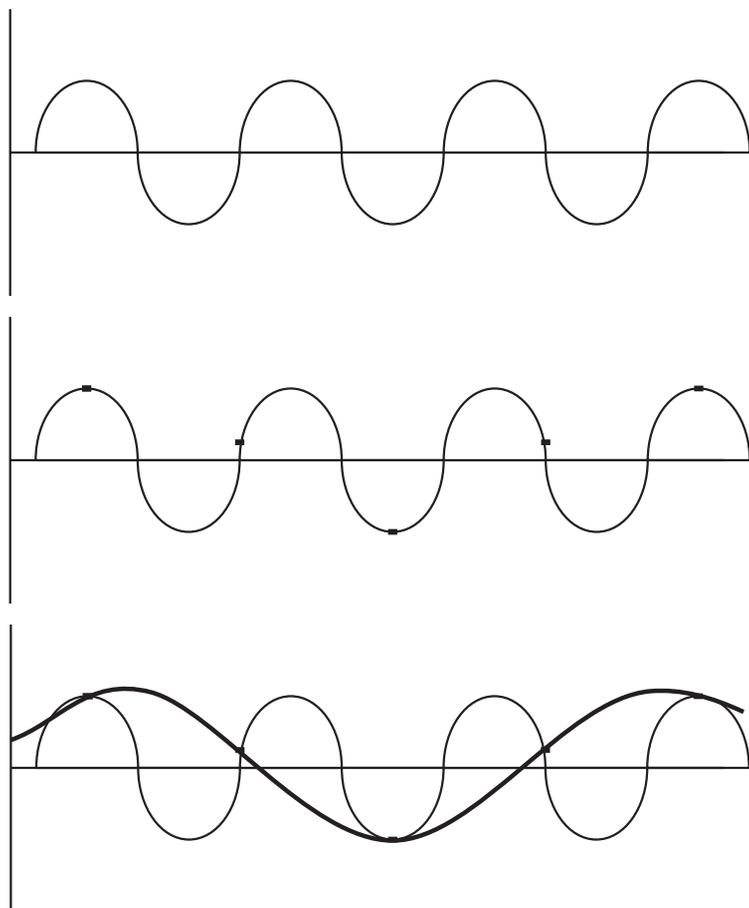
**Figure A.6** Aliasing results when frequencies higher than the Nyquist frequency are sampled digitally. The frequency above the Nyquist frequency “folds over” back into the audio range. When the original frequency (top) is sampled at too low of a rate (middle), the result will be an “artificial” lower frequency that does not exist in the original signal.
