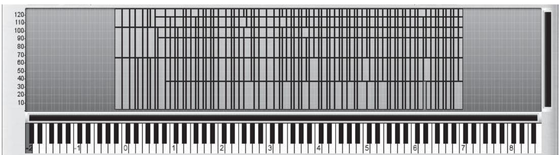
**Figure C.11** The cross-switch function in synthesizers and samplers is used to trigger different programs or samples based on velocity values. In this case, a separate sample has been assigned to each of the key zones, and different samples are played for the zones based on the velocity of the key strikes.
