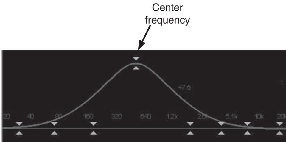
**Figure C.2** Bell filters boost or cut frequencies around a center frequency.
