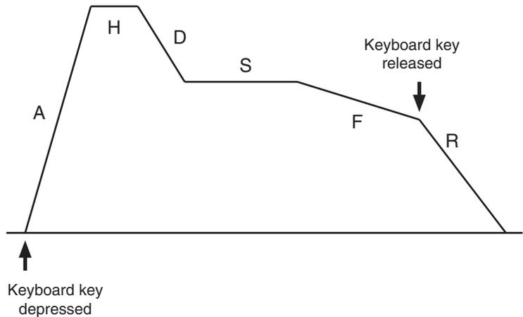
**Figure A.4** An AHDSFR adds hold and fade stages to the standard ADSR envelope.
