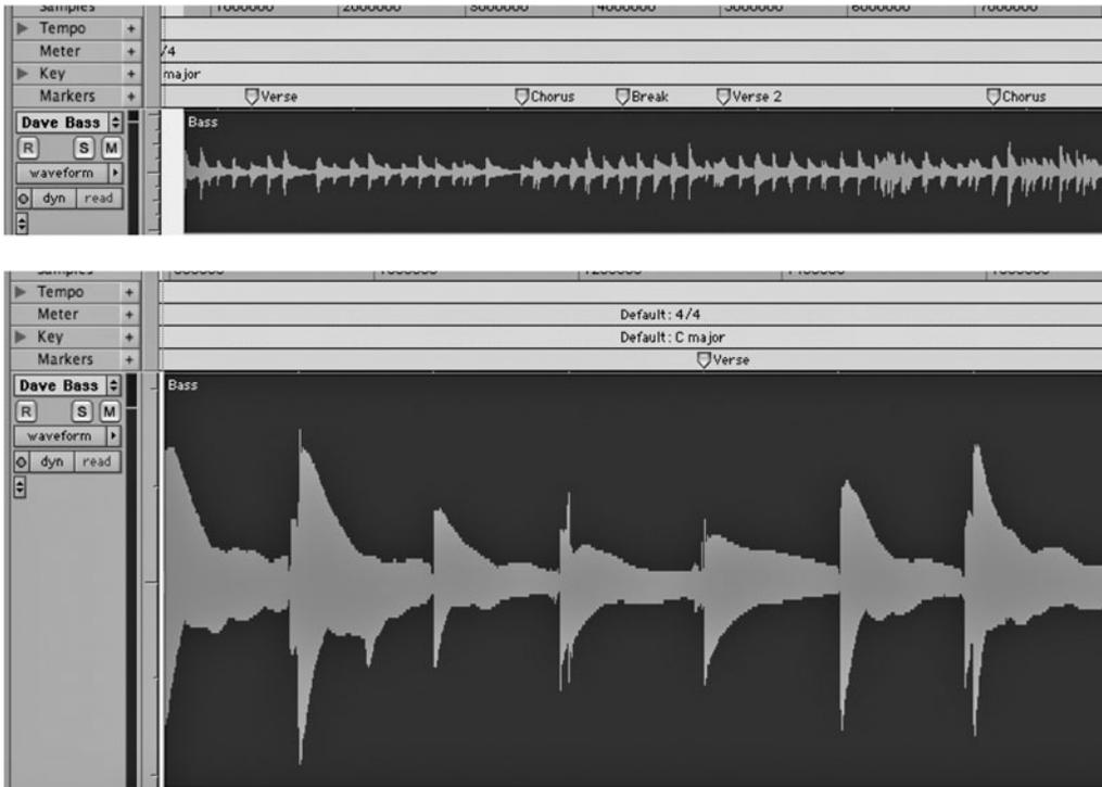
**Figure 2.5** DAW and audio editing programs allow the user to increase the size of waveforms and other displays to allow finer editing. A track can be viewed with a low zoom level (top) to show more of the track, or the view can be zoomed in (bottom) to allow a more detailed view.
