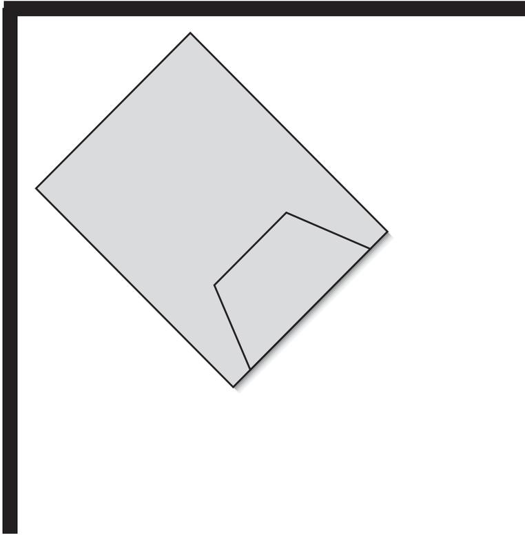
**Figure Q.4** A speaker in quarter space will have a substantial bass boost.
