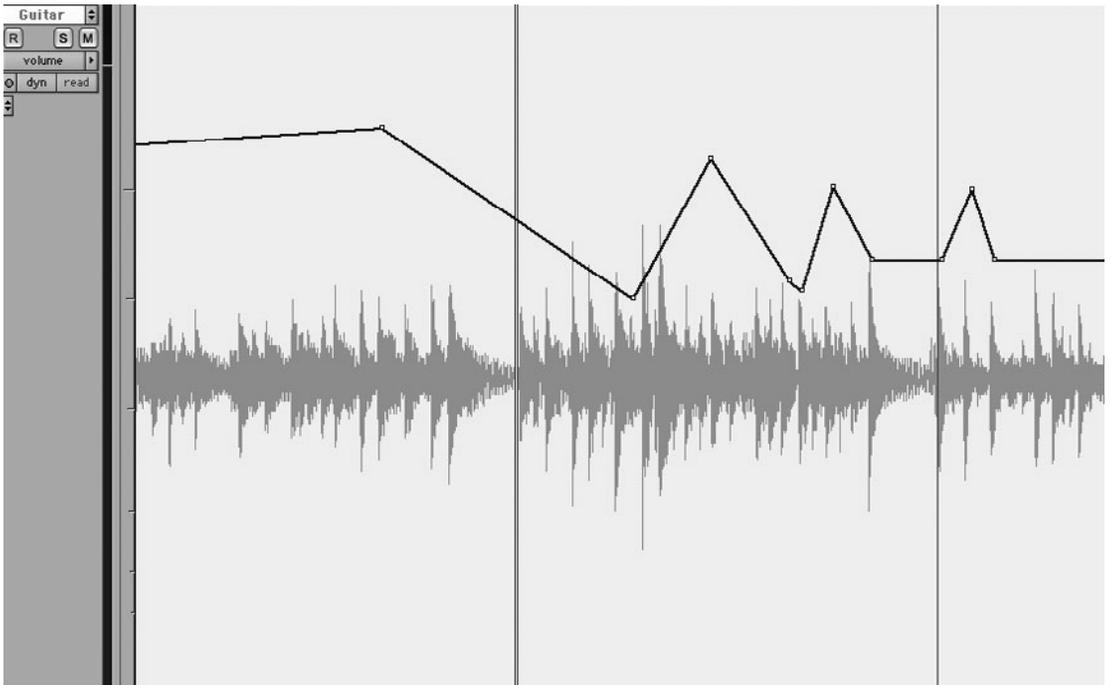
**Figure B.13** Linear automation “curves” are created using data points (called breakpoints) inserted in a track.
