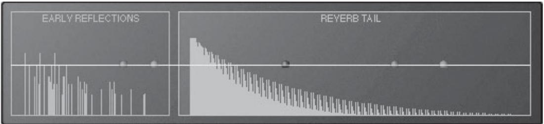
**Figure L.2** The late reflections portion of a reverb is the wash of ambience that occurs after the early reflections.
