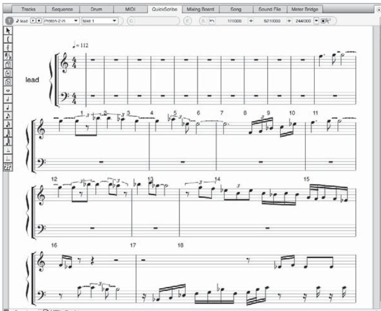
**Figure S.3** The score window in a DAW or sequencer displays MIDI notes as standard musical notation. The notes can be easily edited using a mouse.
