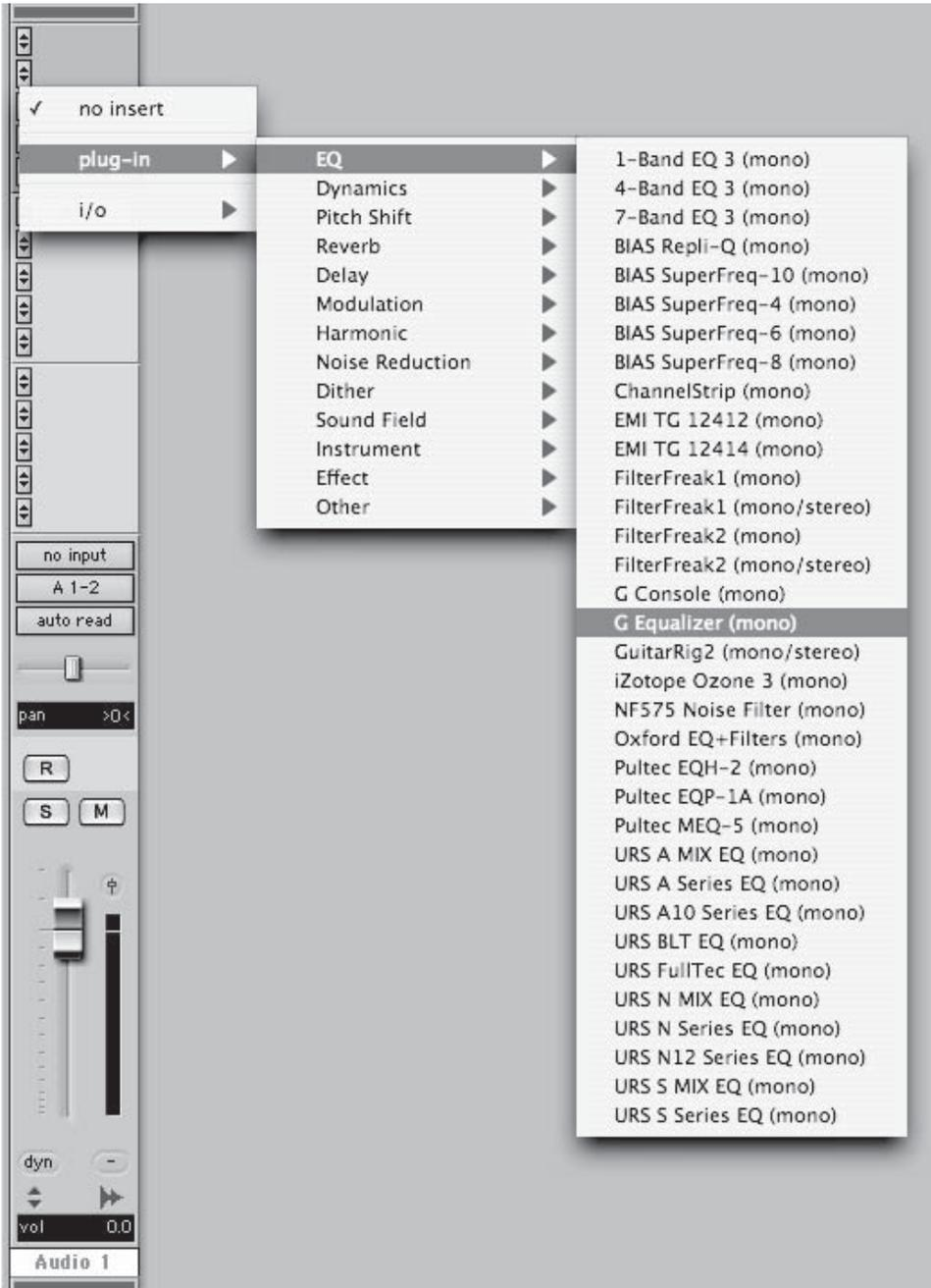
**Figure I.3** DAWs feature insert slots—analogue to insert points in hardware mixers—that can accept plug-in processors.
