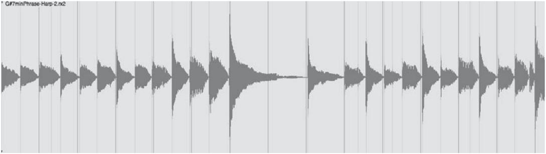
**Figure S.9** In a REX file, the audio is chopped into rhythmic slices so that it can be played back faster or slower or otherwise manipulated.
