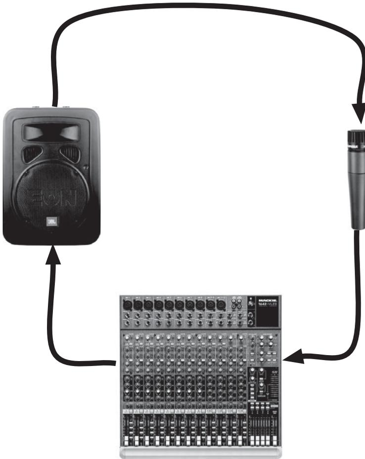
**Figure F.2** Feedback results when a signal loops repeatedly through a device or system, increasing in intensity until it is out of control.
