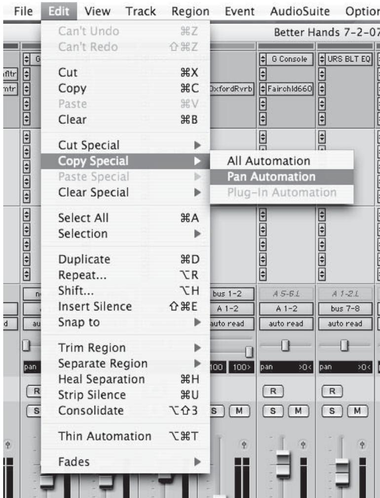
**Figure M.2** A program’s or operating system’s menus organize the available commands into lists. Submenus branch off from the main menu and provide related command options.
