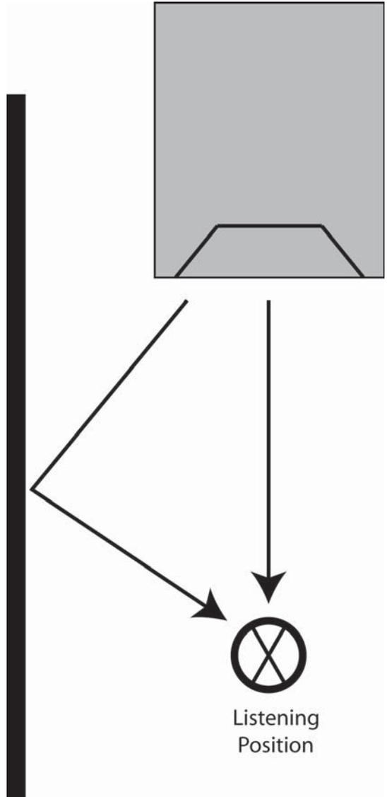
**Figure F.4** A first reflection is a sound wave that reaches the listener immediately after the direct sound, after reflecting off of one surface.
