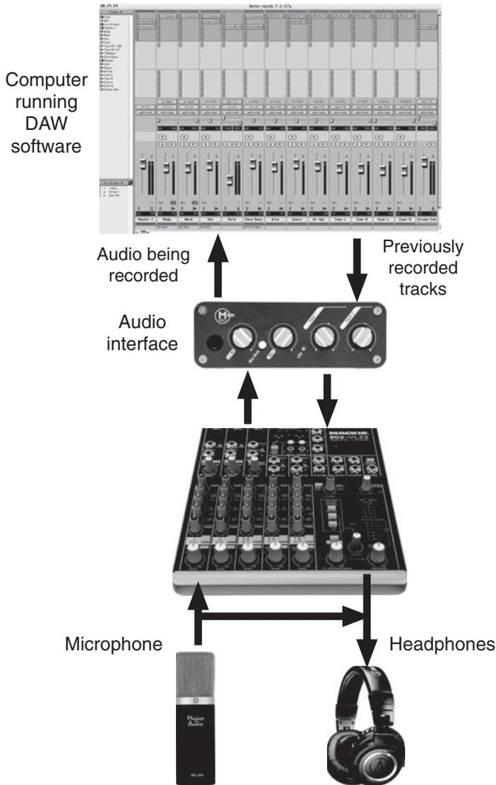
**Figure L.3** A mixer can be used to monitor signals that are being recorded, eliminating the problem of latency when tracking or overdubbing.
