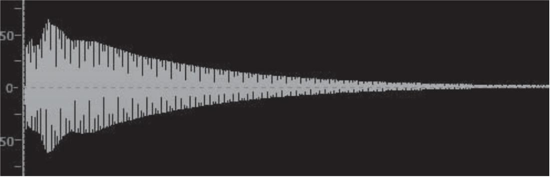
**Figure A.8** Attack refers to the beginning of an event, such as the start of a sound wave or synthesizer note, or where a change in a processor’s response occurs.
