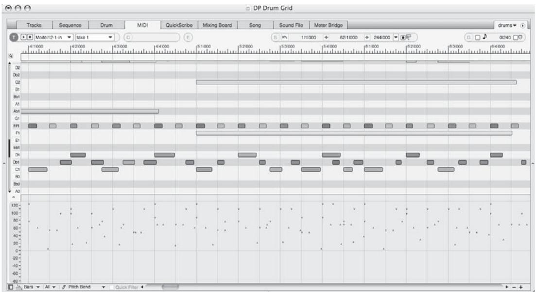
**Figure L.1** A lane is used to display control information related to the MIDI or audio data in a track. In this case, MIDI notes are shown in the top section, while velocities are shown in the bottom lane.
