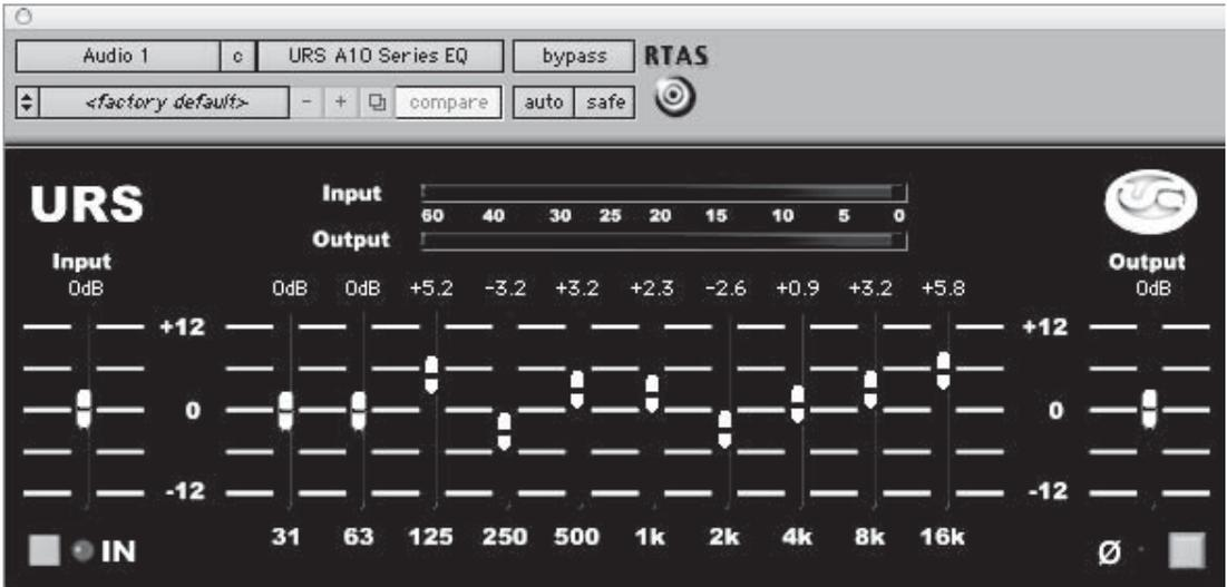
**Figure H.5** Because they resemble bar graphs, certain types of meters are referred to as histograms. In this example, there is a histogram (to the right of the left/right input meters) of the waveform peaks in the input signal.
