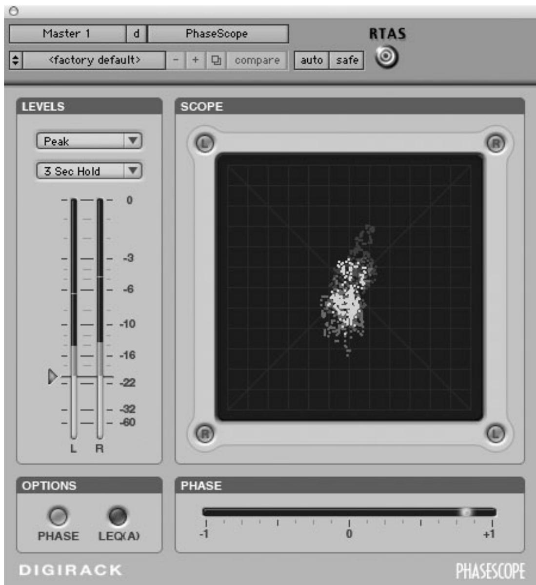
**Figure J.3** Jellyfish meters are used to display information about stereo and multichannel surround audio signals.
