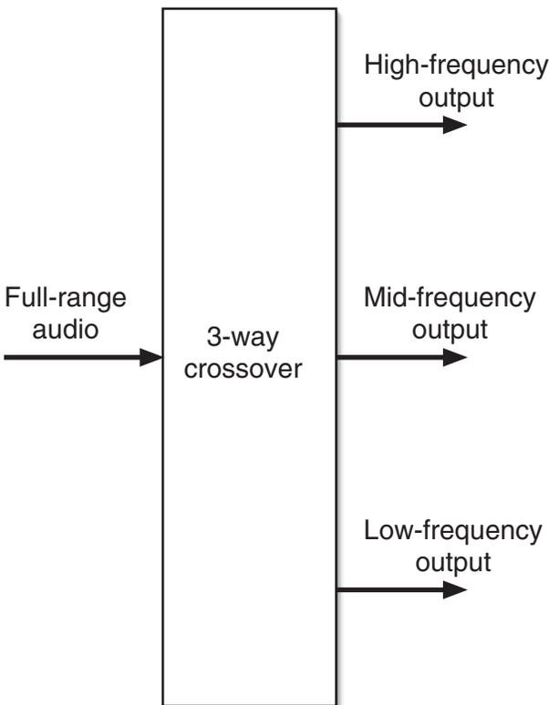
**Figure C.12** A crossover splits full-range audio into two or more frequency bands so those bands can be amplified or processed separately.
