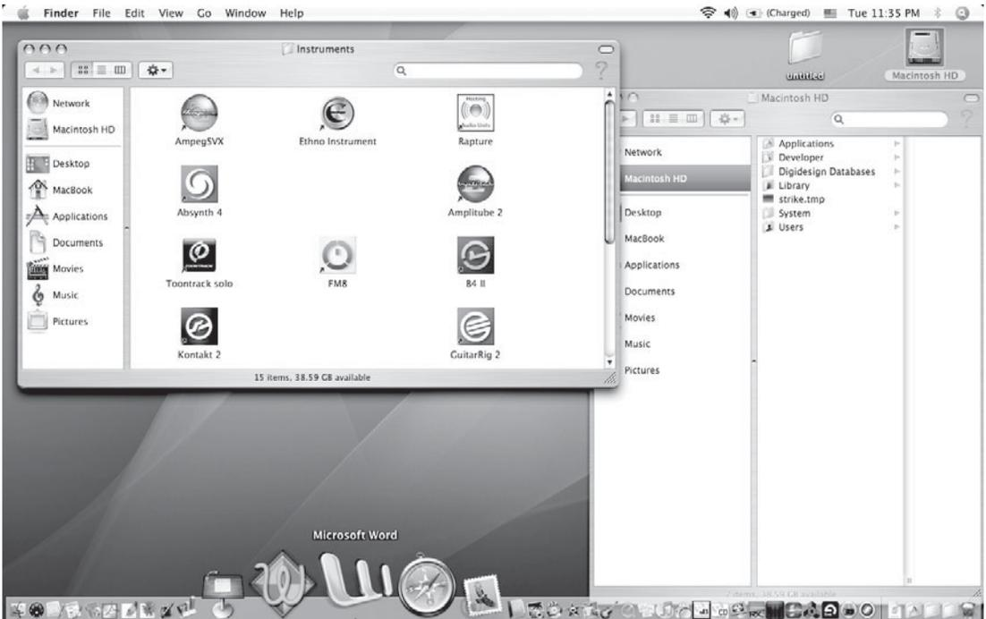
**Figure G.2** A computer's GUI, or graphical user interface, consists of a variety of elements, such as icons, menus, switches, control panels, knobs and other controls, folders, and more.
