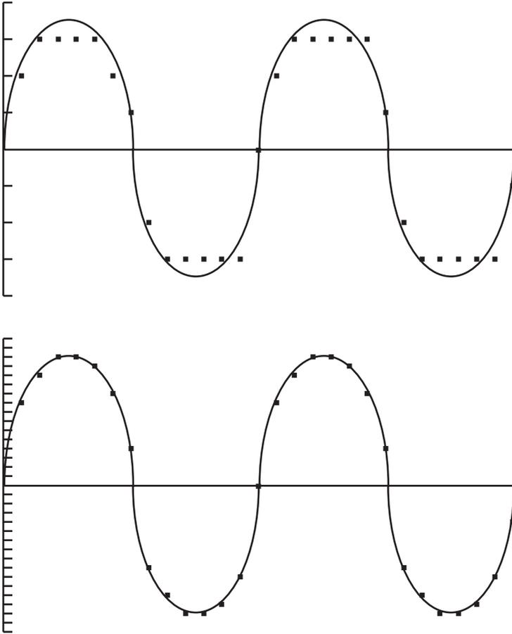
**Figure B.9** Adding more bits to a digital audio system increases the resolution from low (top) to high (bottom), resulting in a more accurate picture of the audio waveform.
