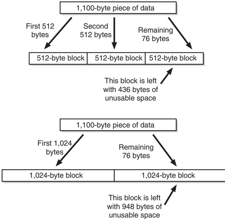
**Figure B.10** A comparison of how data block size can impact how much data can be stored on a disc or drive—the larger the block size, the more space is wasted.
